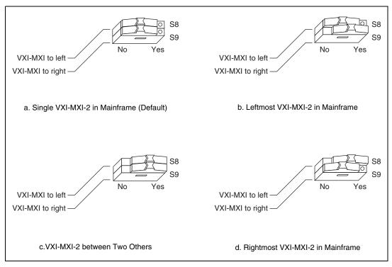
Figure 3-4. VXIbus Local Bus Configuration
